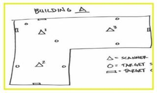
Move Scanner to Next Station. For Best Results Keep Stations within 20-30m for Interiors and 10m for Exteriors.
