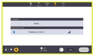
Connect Tablet to Scanner Via WIFI or Cable. Using WIFI, If Scanner doesn't Populate than Tap "Find".
