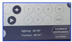
Fine Tune Instrument's "Sighting" and "Trunnion". As Close to All Zero's as Possible.
