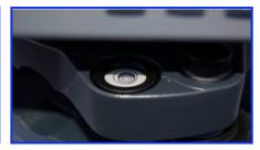
3 Level Instrument Using Tribrach Bubble.
