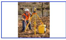
2 Set Tri-pod Legs Clear of Obstruction. 24-30" From Center of Instrument
